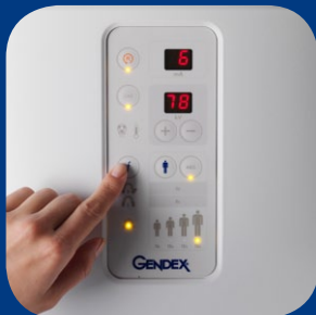
Intuitive control panel for simple setup of panoramic and TMJ projections
